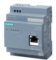
LOGO! CSM12/24 Compact Switch Module connection of a LOGO! (...0BA7/...0BA8) and up to 3 further nodes to Ind. Ethernet with 10/100 Mbit/s Unmanaged switch, 4 RJ45 ports, 1x front port for diagnostics DC 12/24V power supply LED diagnostics, LOGO! setup.
